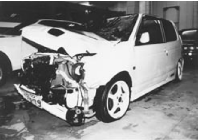
FIG. 1—The damaged front end of the car after salvaging from the sea.
